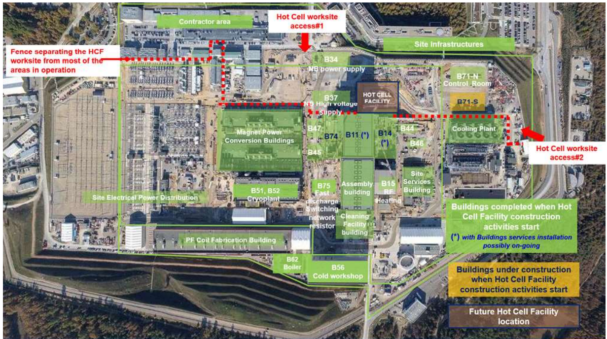
Figure#2: Site Layout with location of the Hot Cell Facility Worksite area 5 .
